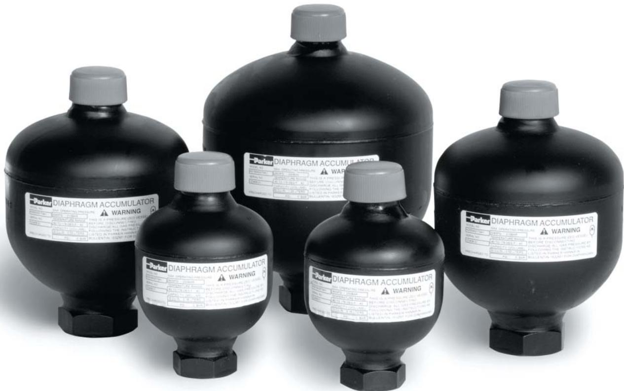
Diaphragm accumulators provide an affordable means of enhancing the performance of a hydraulic system. They are suitable for storing energy under pressure, absorbing hydraulic shocks, and dampening pump pulsation and flow fluctuations.
