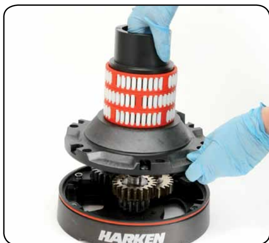
11. Remove the drum support n°16
