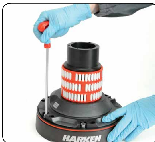
10. Unscrew the 6 hex screws n°17 ( 20Nm/177 in-lb)
