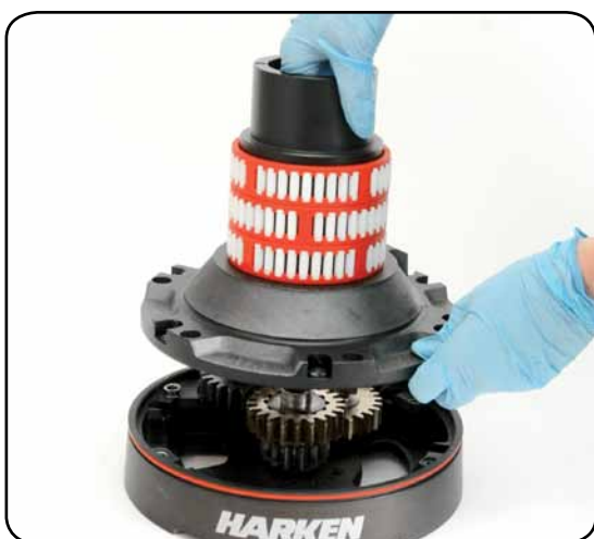
11. Remove the drum support n°16 Important: washer n°7 may remain inside the drum support!
