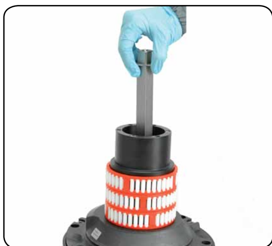
9. Slide out the central shaft n°19
