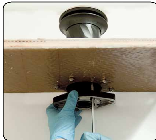
2. Tighten the six screws (⚙️ 8 Nm/ 71 in-lb)
