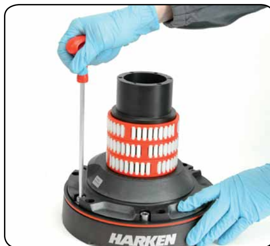
10. Unscrew the 6 hex screws n°17 ( 20Nm/177 in-lb)
