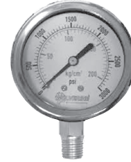
2-1/2" Round Face, Stainless Body, 1/4" NPT (Male Brass Fitting), Dual Scale (PSI & kg/cm 2 ), Lower Mount.
