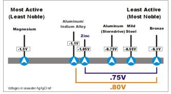
In order to provide protection, the highest practicable voltage difference possible is required between the sacrificial anode and the metal to be protected. For example, if zinc is used to protect a bronze propeller, a "driving or protecting voltage" of negative -0.75 volts will be available, i.e. zinc at -1.05 volts minus bronze at -0.3 = -0.75 volts.
