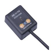
ZCC211S-JQR is a plane digital module with low cost. It sends dada via232.It features high accuracy and Stable performance. Output baud rate is 9600bp/s.
